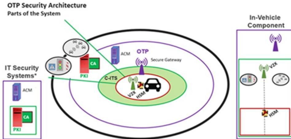
**Figure 13: Example of a layered OTP security architecture containing an enhanced, secure gateway that controls and secures the dataflows to and from the vehicle**
