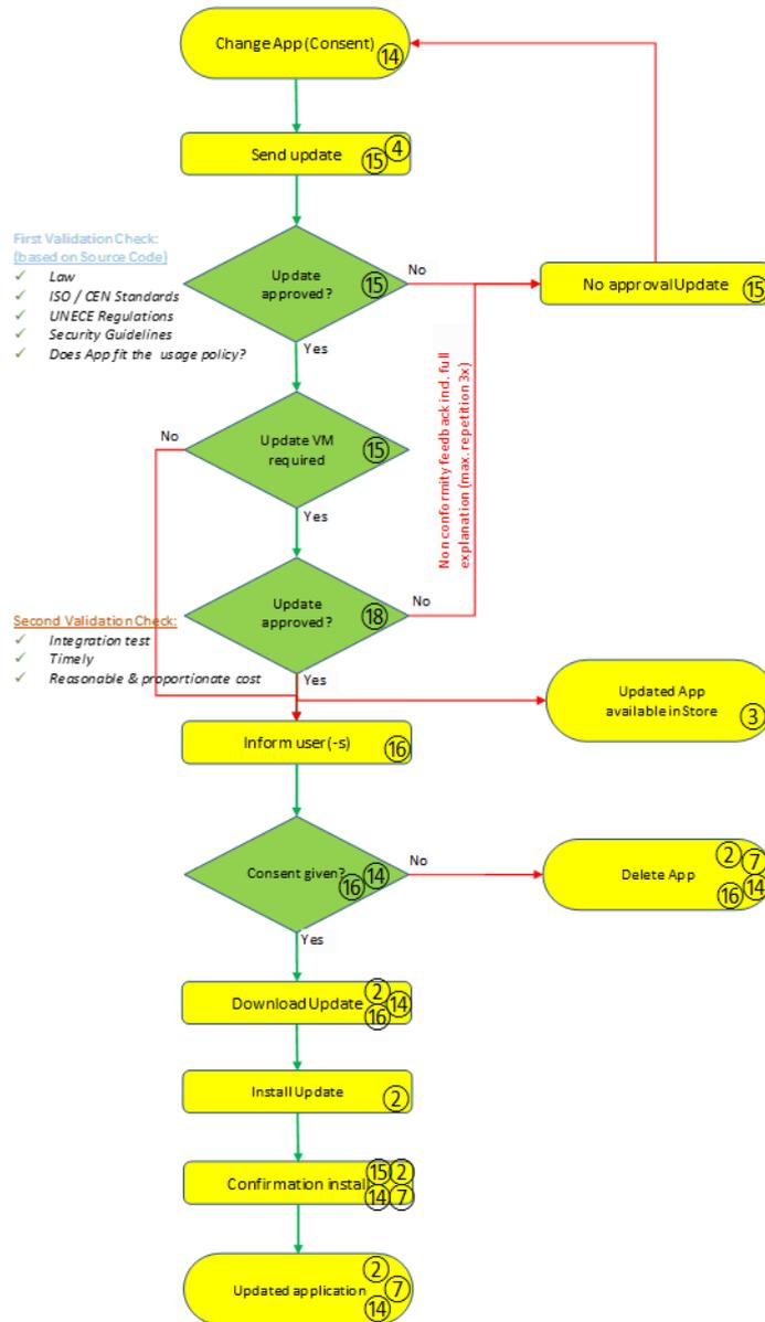
Figure 29: Process for change of vehicle owner consent
