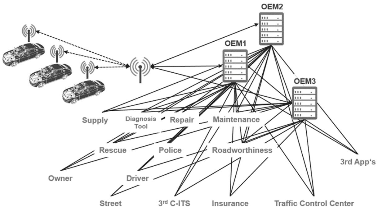
**Figure 10: "Wired" 'Extended Vehicle' scenario for Car2X communication**
